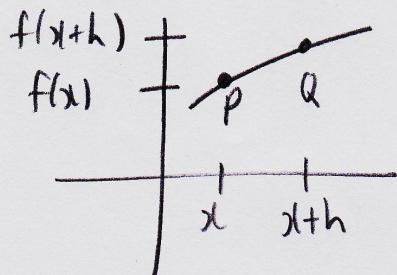
$$\begin{aligned} \text{Slope of } PQ \quad m_{PQ} &= \frac{\text{rise}}{\text{run}} \\ &= \frac{f(x+h) - f(x)}{(x+h) - x} \\ &= \frac{f(x+h) - f(x)}{h} \end{aligned}$$
